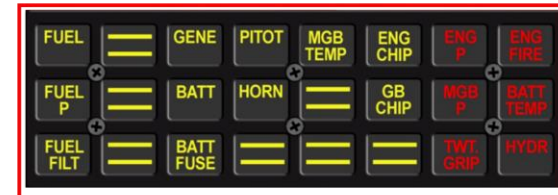
Caution and Warning Panel (CWP)
