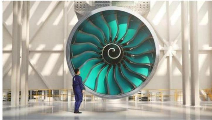
The Trent UltraFan will be 25 per cent more fuel efficient than its 1990s-era predecessor. It does so by being very big - its diameter is slightly smaller than that of a London Underground tunnel - and shifting more air through a larger fan, improving efficiency. Photo: Supplied
