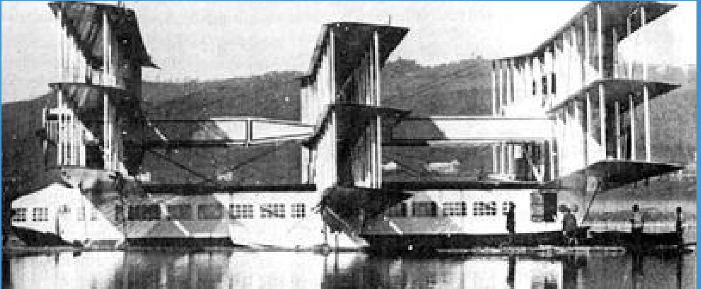
The **Caproni Ca 60 Noviplano**, dubbed the 'Capronissimo', was an absurd aircraft which featured three sets of triplane wings set above a giant fuselage which resembled some sort of luxury houseboat.
