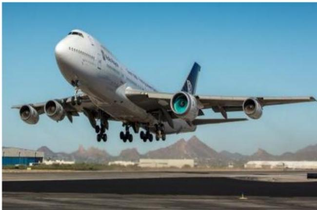
*The Ultrafan engine dwarfs the regular engines on a testbed Boeing 747. Photo: Jonathan Green*
