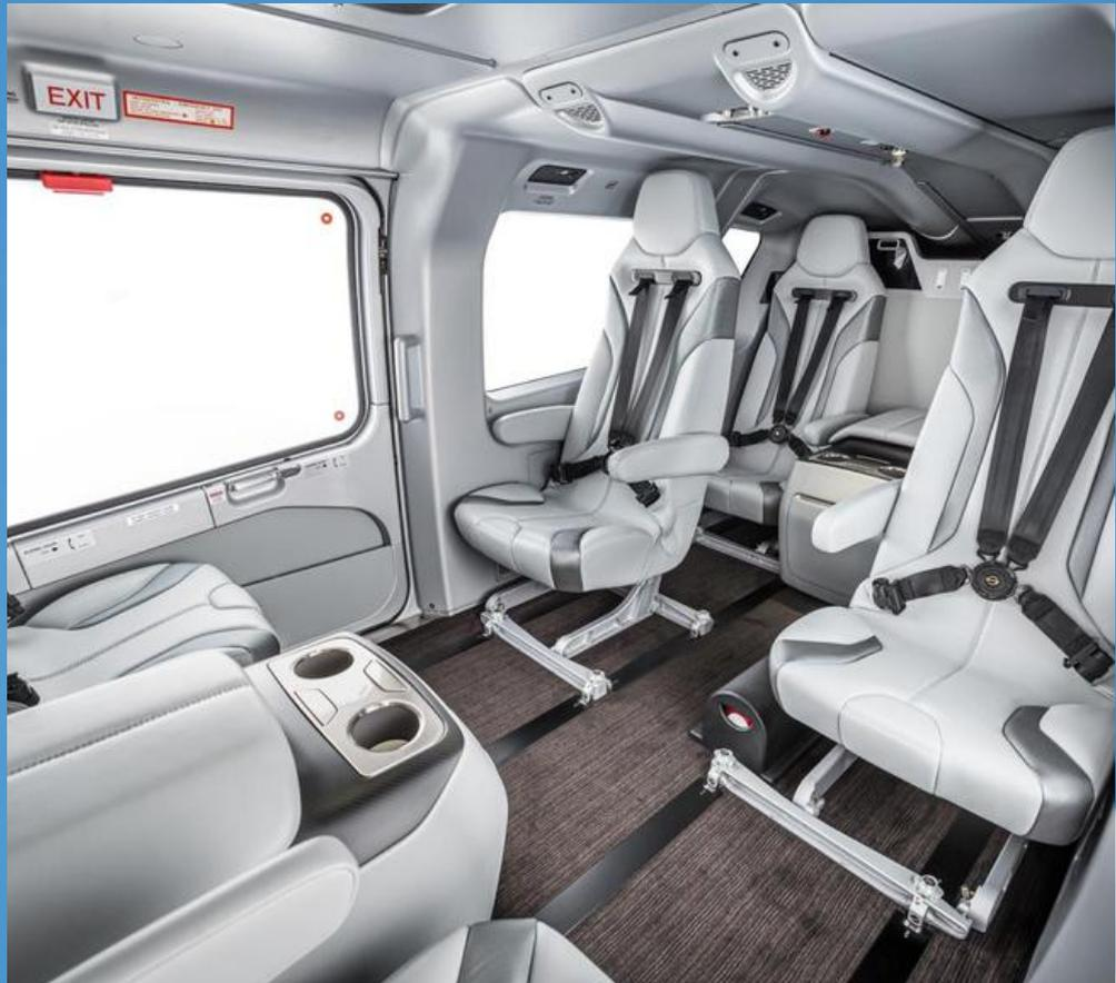
Its cabin is fitted with ACH's clean and modern ACH Line interior configuration in a grey theme but the leather elements essential to its luxury feel are replaced with Ultraleather which captures the visual and tactile leather experience with comparable durability.
