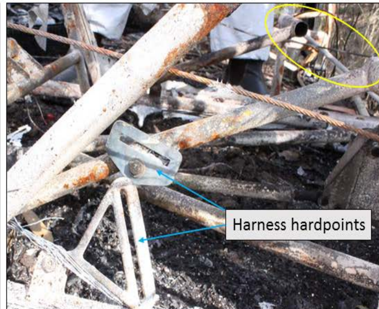
Rear crotch strap hardpoint - missing
