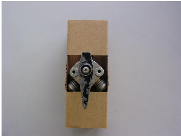
Position of the selector as found on ZK-JGI.
