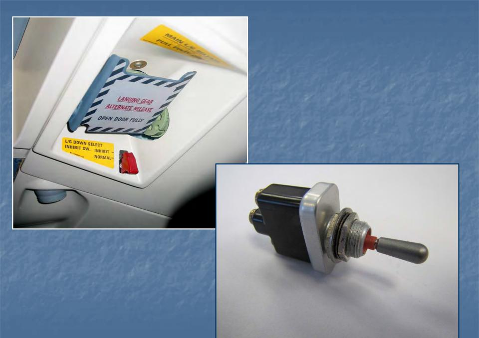
This was also cause of nose wheel steering defect at HLZ. Both systems get hydraulic pressure when the gear is selected DOWN
