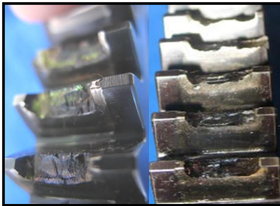
Main Accessory Gear Damage
