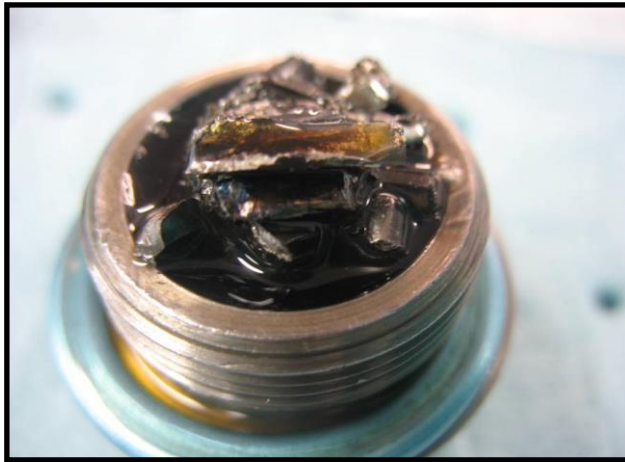
Magnetic Chip Detector Debris (Post Failure)
