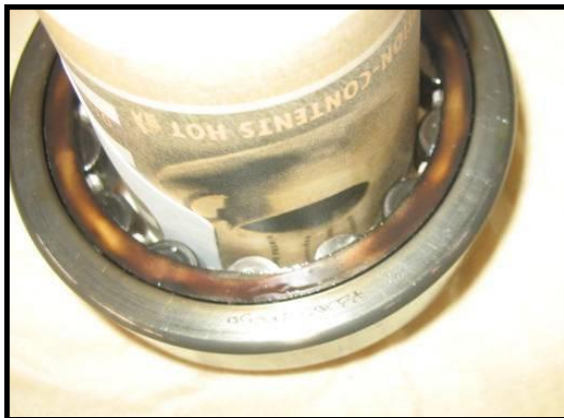
Bearing Cage Heat Damage
