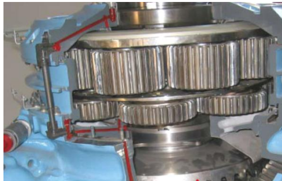
Eurocopter AS332L2 Super Puma main gearbox epicyclic gear set
