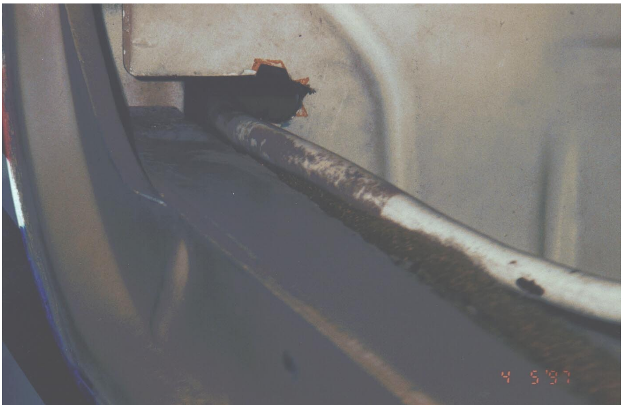
The hose running into the cabin was not restrained, nor protected from chafing, or cutting.
