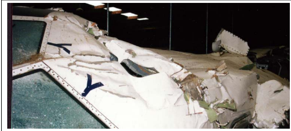
Figure 18. View from front of fuselage, showing crush lines and ingrained dirt.
