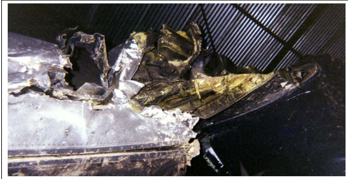
Figure 23. Damage to upper skin of starboard tailplane. The square hole has extensive sooting inside; the deflection damage has very little sooting.
