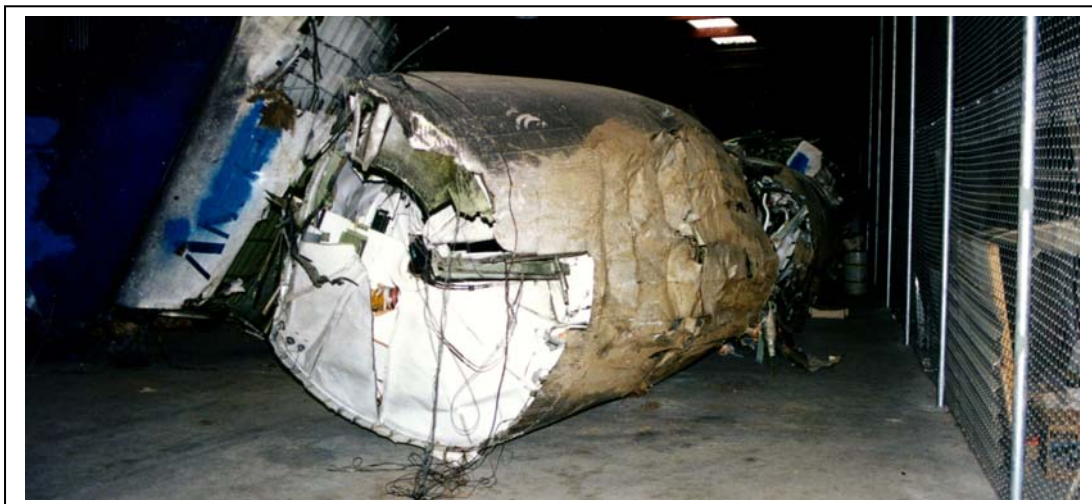
Figure 21. View from bottom rear of fuselage. Impact damage is ahead of rear bulkhead. Note flattening at top of rear fuselage.
