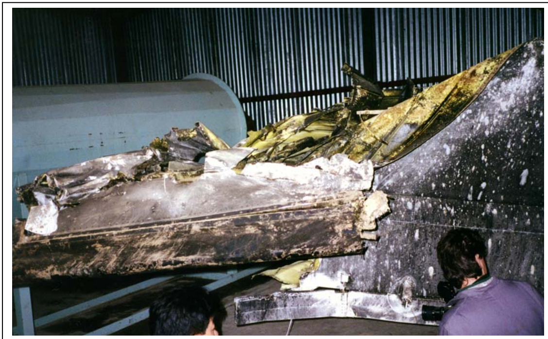
Figure 24. Damage to leading edge of fin and upper surface of tailplane. There was no corresponding damage on the outer portion of the right wing. Soot deposits around rivets are fairly even, suggesting static fire.
