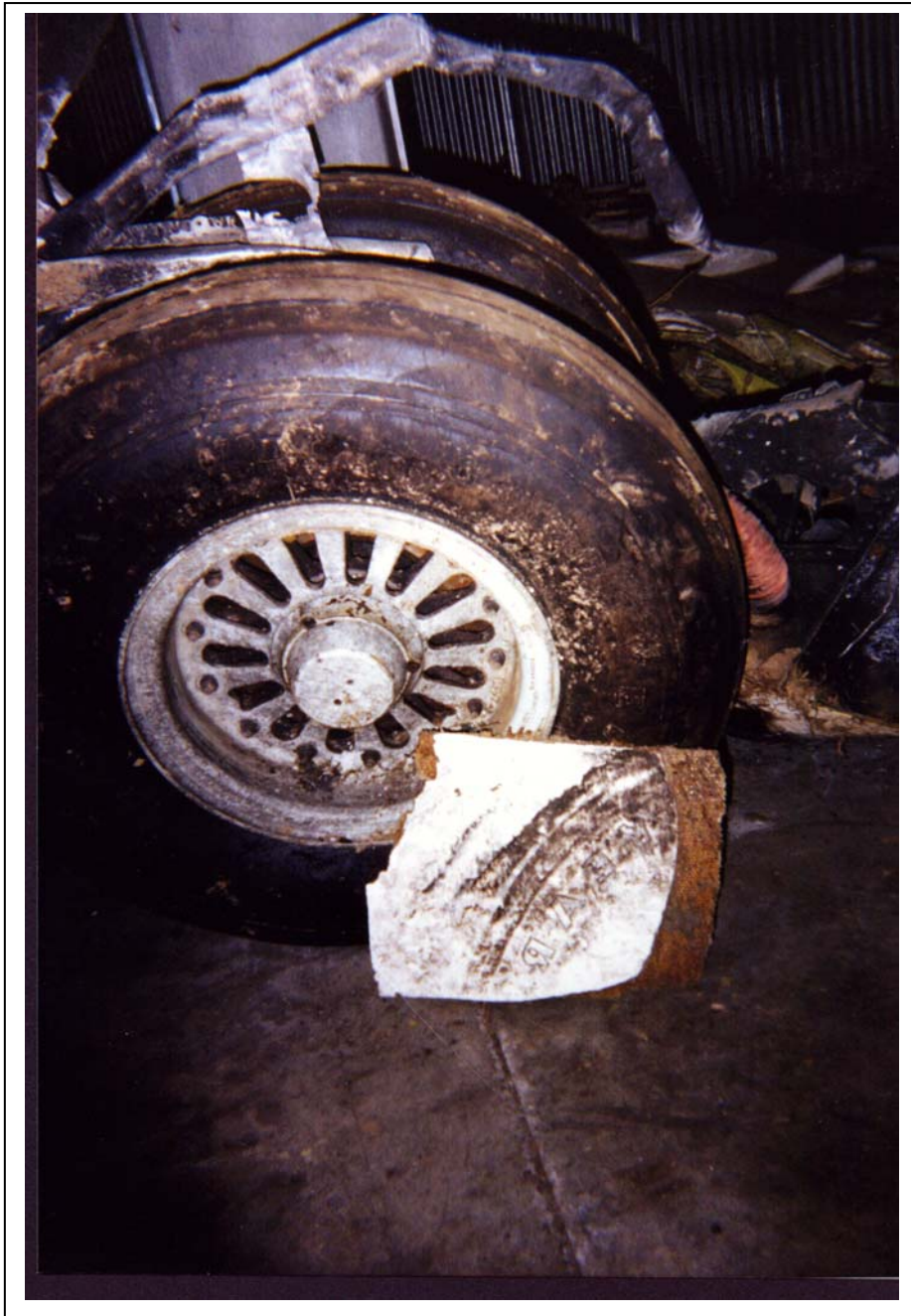
Figure 17. Witness mark on part of right hand undercarriage door.
