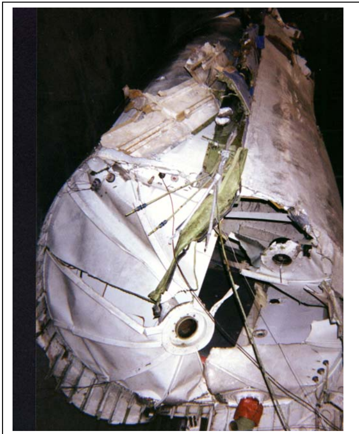
Figure 19. View from rear of fuselage, showing crush line, and torsional damage to rear bulkhead.
