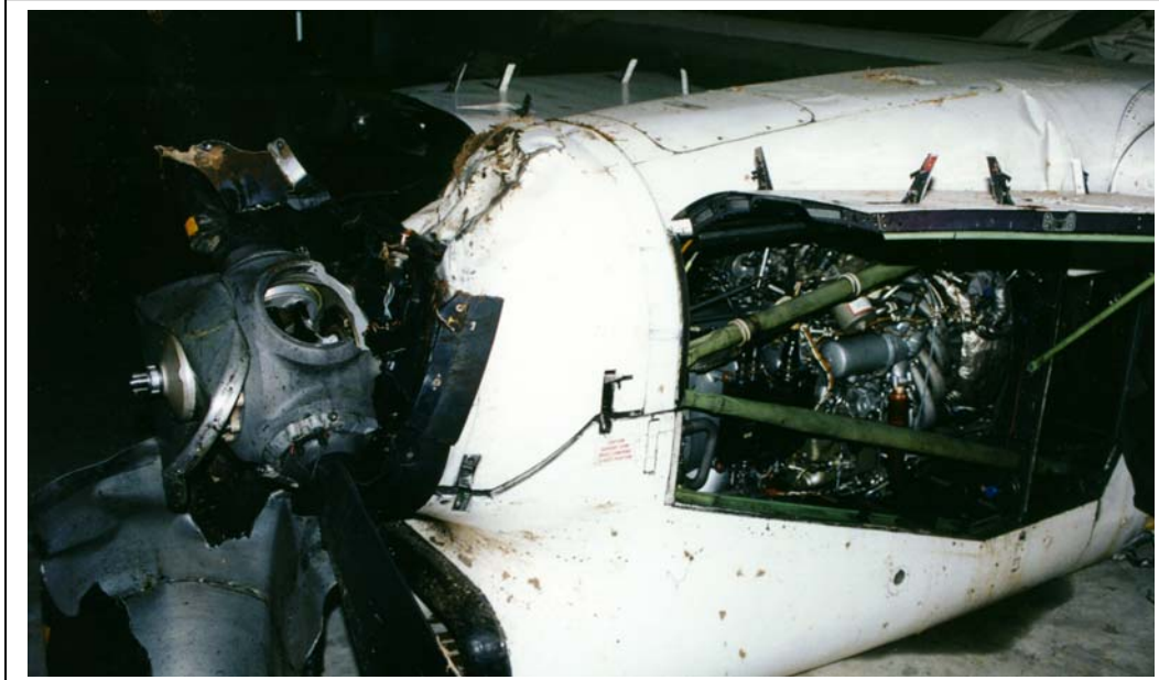
Figure 20. Left engine nacelle, showing lack of damage to underside, and inverted ground contact. Damage to the propeller shows that it was in this position, and rotating, when the nacelle struck the ground.
