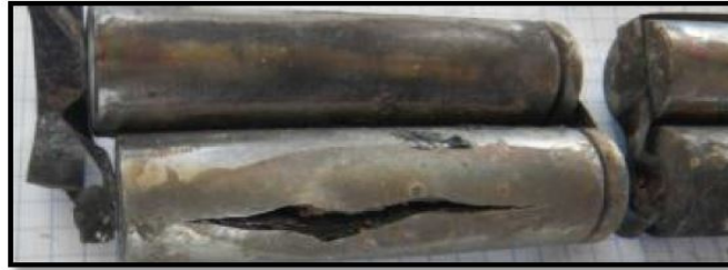
Fire damaged remains of battery pack with a fractured cell
