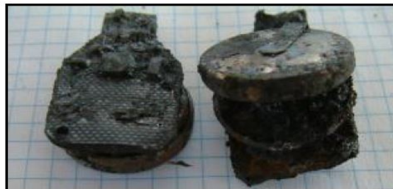
Lithium primary button sized flat cell batteries (watch style) with small circuit board
