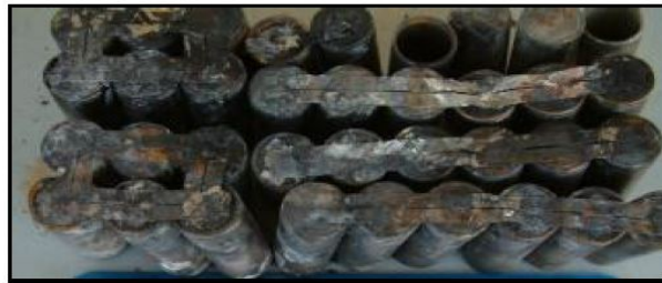
36-cell lithium-ion battery pack with multiple vented cells
