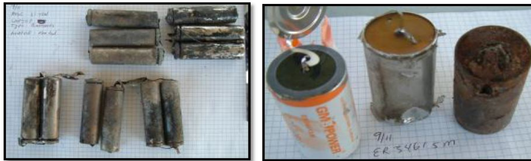
Additional battery pack remains [LH]/D-Cell size lithium primary batteries. Photo shows fire damaged and undamaged batteries [RH]
