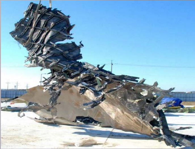
Burnt through skin panel (Photo: ARAIB)
