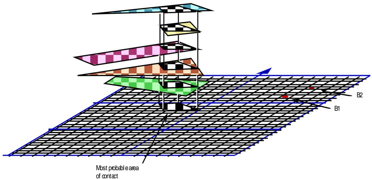
Figure 6: Most likely location of impact (grey shaded area). Each other colour represents the estimated projection of a component group (separated in height dimension for illustration purposes).
