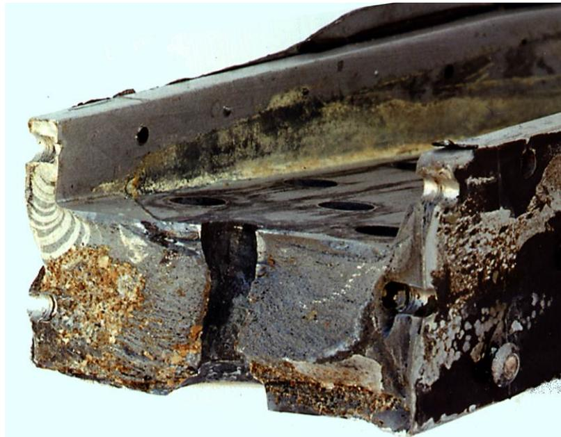
**Figure 7: Fracture surface of A7-076 lower spar cap after recovery from the ocean. Note the fatigue progression marks propagating from the upper (nominally) blind fastener hole (upper left hand side).**
