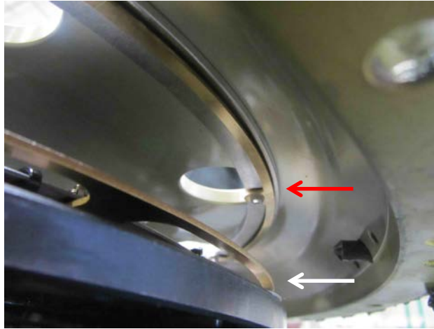
Figure 6. Coils in position before rejoining top cover (static coil red arrow, moving coil white arrow)
