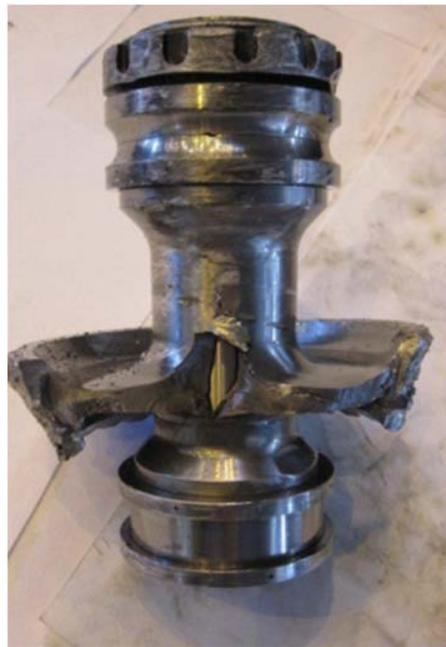
Figure 4: GE90 Transfer Gearbox Pinion Gear
