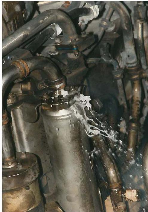
Figure 6: CF6 Wet Motor Leak Test
