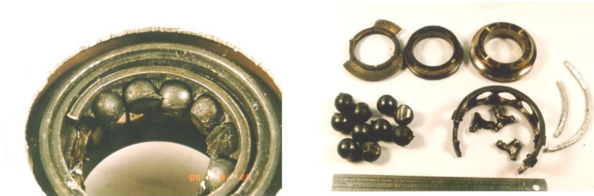
Figures 1 & 2. Destroyed main shaft bearing as recovered
