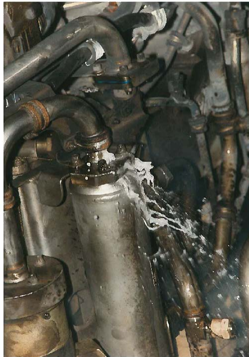
Figure 6: CF6 Wet Motor Leak Test
