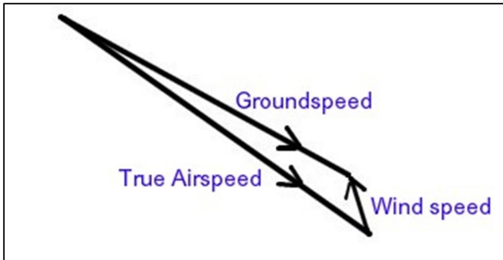
Groundspeed and track are directly determined by the inertial part of the ADIRU while true airspeed is determined from the directly-sensed parameters computed airspeed, total air temperature and pressure altitude. Wind speed and direction are then indirectly derived as the difference vector between groundspeed/track and true airspeed/heading.
