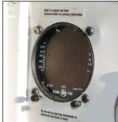
The EDM 700 has a non-volatile long term memory for engine trend monitoring purposes. If the instrument is set to record, it will store all the information displayed once every six seconds or at a programmed interval between two to five hundred seconds.
