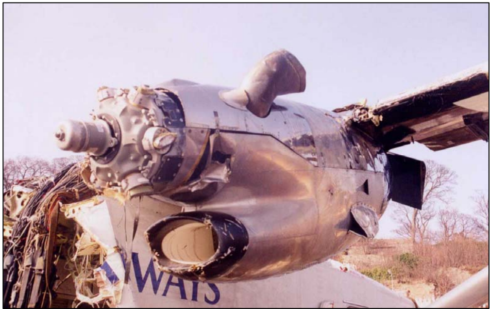
Figure 6: Left engine nacelle with external intake and one exhaust stack visible after wreckage recovery
