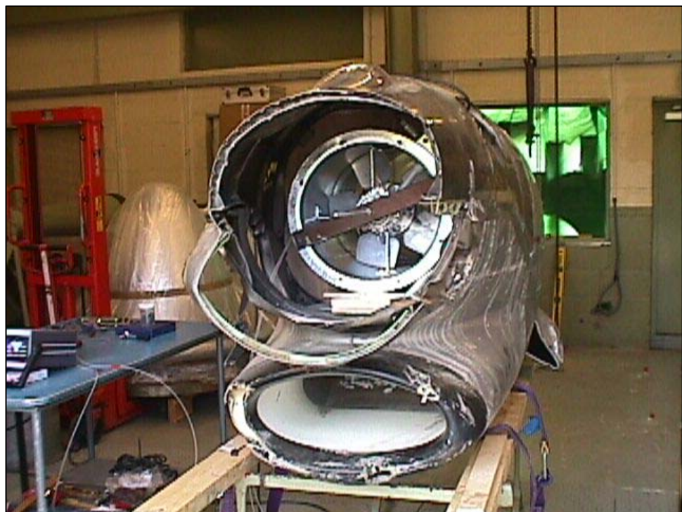
Figure 6: Left engine nacelle with external intake and one exhaust stack visible after wreckage recovery
